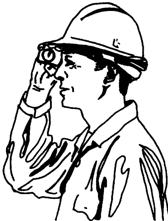
Figure 4-8. Estimating slope with a clinometer.
